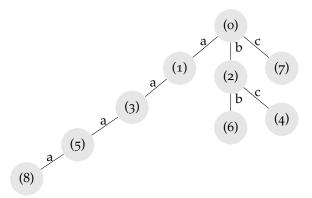
The digital search tree for the Lempel-Ziv code associates one "piece" with each node, starting with the piece "o" as the root. The edge values seen on the path from the root to piece "i" describe the symbols of piece "i". Thus, if piece "i" is the concatenation of piece "j" and symbol S, then j is the parent of i in the DST, and the edge value of (i, j) is S.
